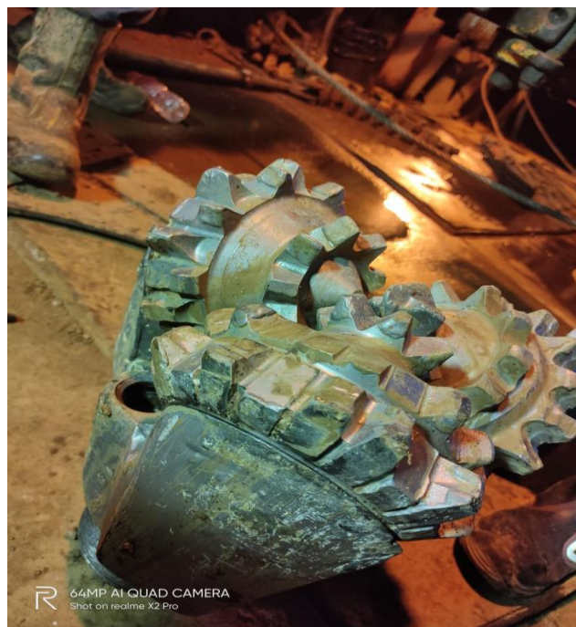
Fig. 5. Photo of 12 1/4" Drill Bit Taken at the Surface
