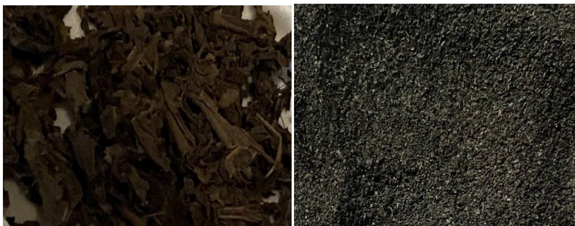
Fig. 1. Tea Waste before and after Carbonization and Activation
