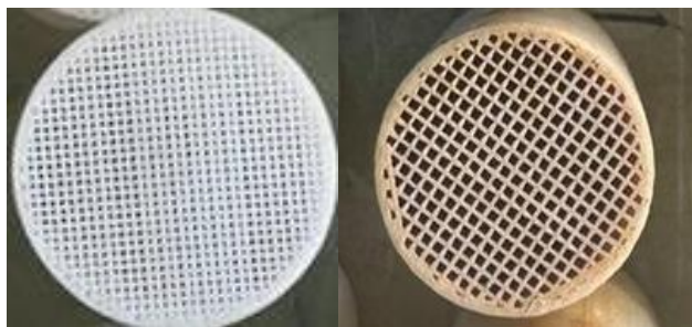
Fig. 1. 3D Printed and Coated Filter by Iron oxide
