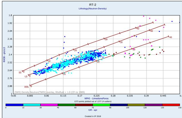
Fig. 3. Neutron-Density Cross Plot for Logs in Well RT-2
