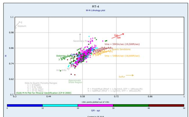
Fig. 9. M-N Plot for Logs in Well RT-4
