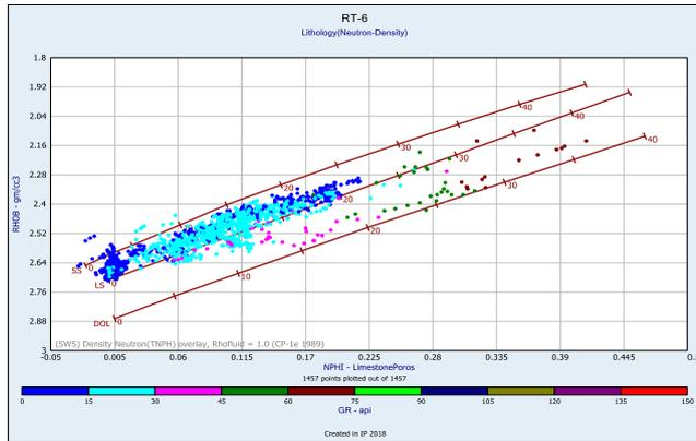
Fig. 6. Neutron-Density Cross Plot for Logs in Well RT-6
