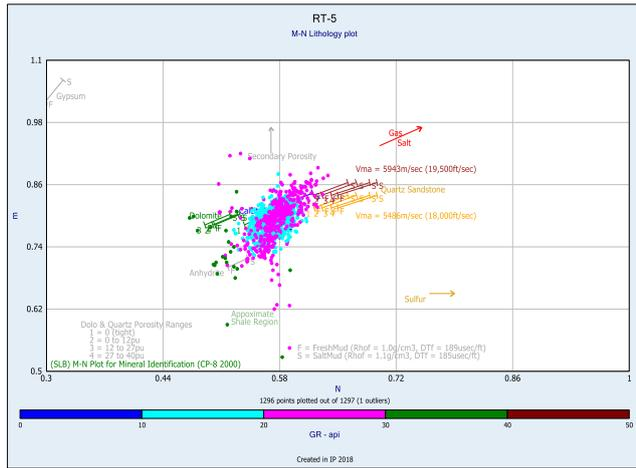
Fig. 10. M-N Plot for Logs in Well RT-5
