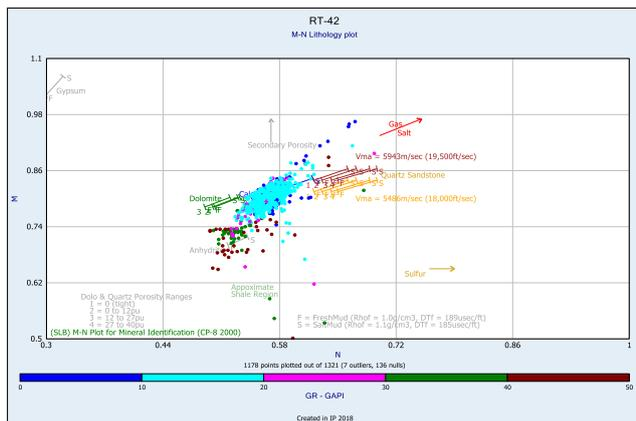
Fig. 12. M-N Plot for Logs in Well RT-42
