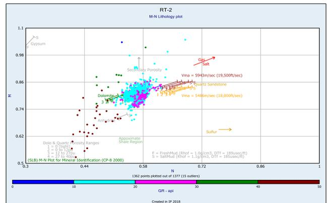
Fig. 8. M-N Plot for Logs in Well RT-2
