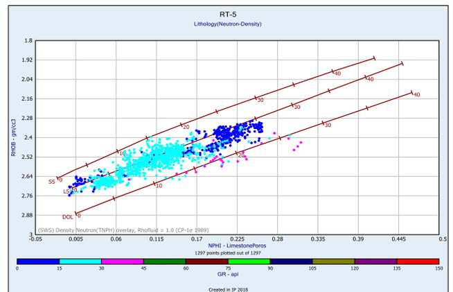
Fig. 5. Neutron-Density Cross Plot for Logs in Well RT-5
