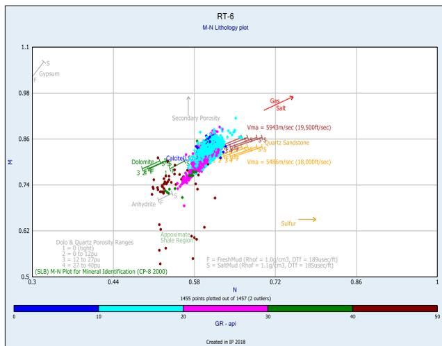
Fig. 11. M-N Plot for Logs in Well RT-6
