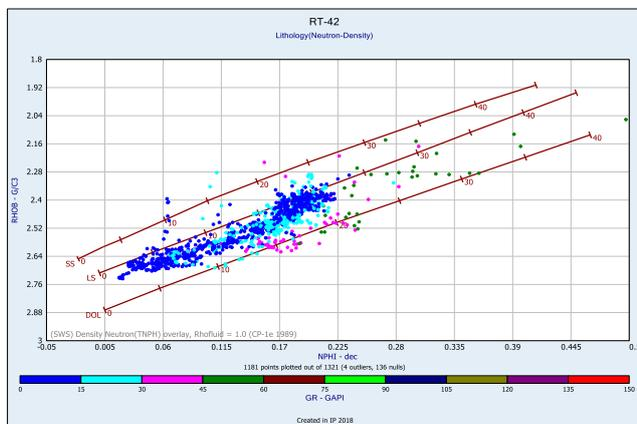
Fig. 7. Neutron-Density Cross Plot for Logs in Well RT-42
