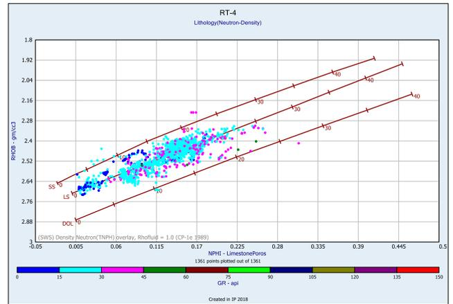
Fig. 4. Neutron-Density Cross Plot for Logs in Well RT-4
