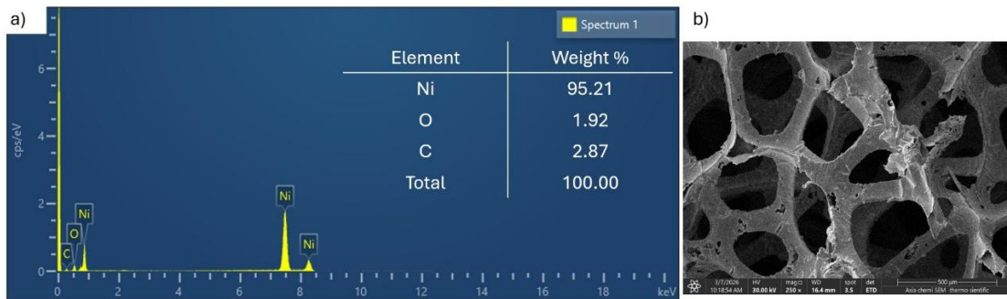
Fig. 8. a) EDX and b) SEM of Ni Foam after using as cathode in EF system
