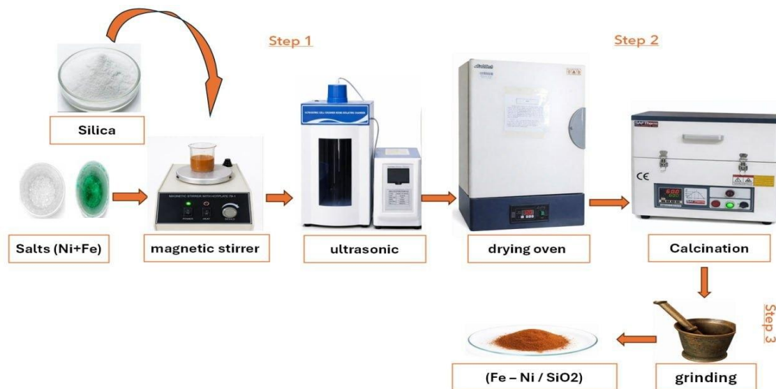
Fig. 1. Preparation of catalyst ( \text{Fe}_2\text{O}_3 - \text{NiO} / \text{SiO}_2 ) by the impregnation method
