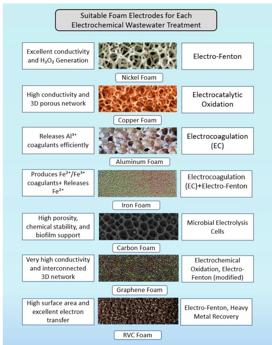
Fig. 6. Summarized the important and efficiency of foam electrodes in the electrochemical treatment for wastewater synthesized from the findings of the reviewed literature (2015–2025) (created by the author)
