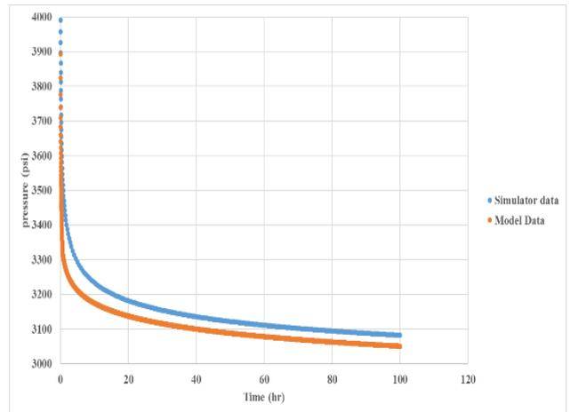
Fig. 7. Bottom hole pressure calculation against simulator results
