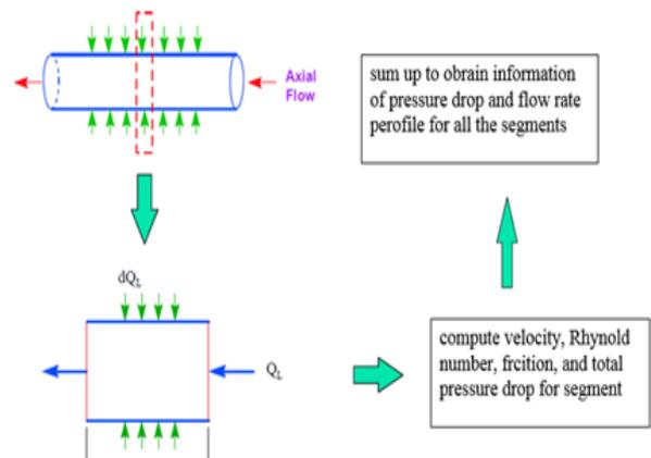
Fig. 4. Illustration of the iterative pressure drop computation [9]
