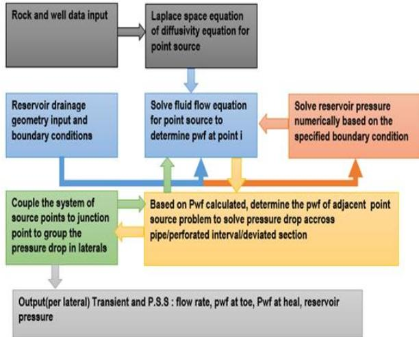
Fig. 5. Conceptual schematic of Python code
