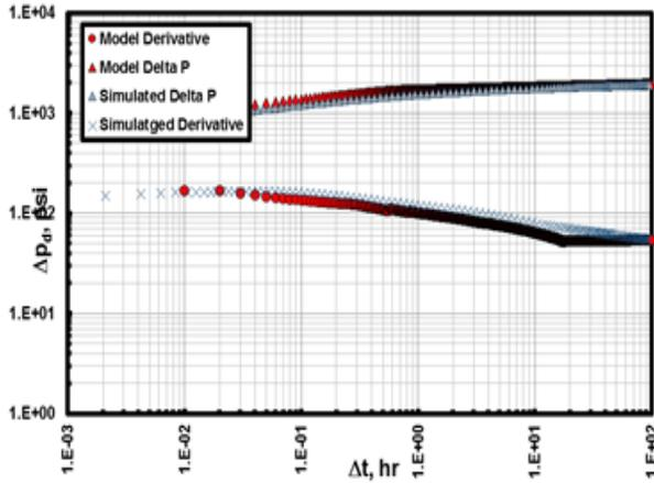
Fig. 8. Pressure drop and derivative log-log plot in comparison with simulated data
