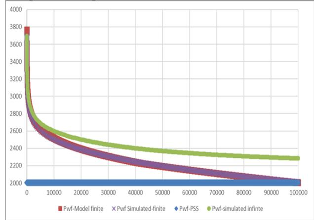
Fig. 13. Comparison of pressure drop between simulator and model
