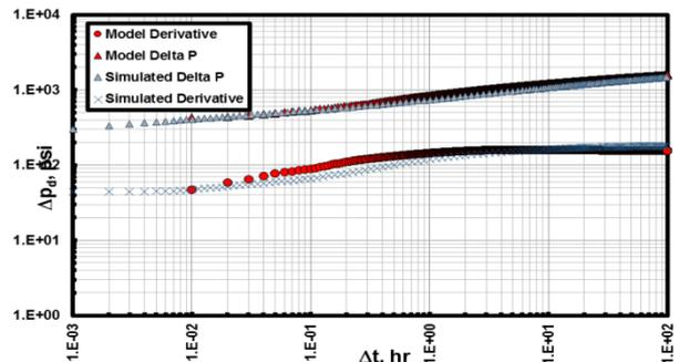
Fig. 11. Pressure drop and derivative log log plot in comparison with simulated data
