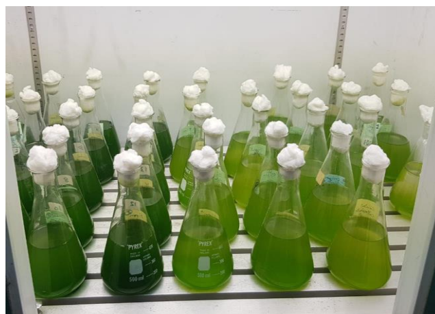
Fig. 1. Microalgae Farms after Added 50 ml of Carbon Dioxide to Culture Medium Concentrations (5, 15, 25, 35) mg/l and a Control Group with Light Intensity 168 \mu\text{Em}^{-2}\text{s}^{-1} and an Ambient Temperature (24 \pm 1 °C )
