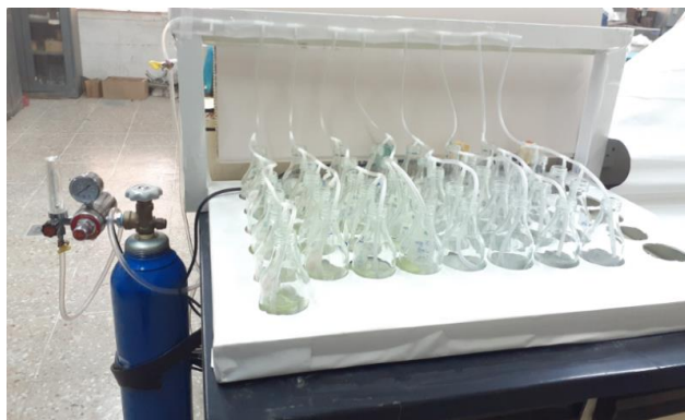
Fig. 2. Screenshot of the Experimental Set-Up Used in the Current Study (Sparging Carbon Dioxide Gas into 50 ml of Microalgae Culture Medium for 5 min with a Flow Rate 2 L/min at Room Temperature)
